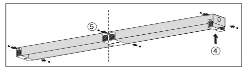
4. Bend brackets to fit the original fixture housing. For RXL-8, make sure centre bracket aligns with the centre of the strip housing length.
