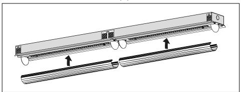
9. Start on one end and slide lens into lip of end cap. Squeeze lens until the lip is under the tabs of the gear tray (it might be necessary to gently push the end cap outwards for the lens to slide into.) To ensure lens is locked in place, gently press the face of the lens.
