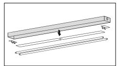
2. Remove original lamps, ballast cover, and sockets.
