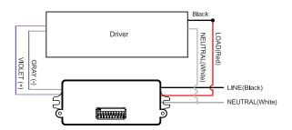
Wiring with non-dimming ballast or LED driver.
