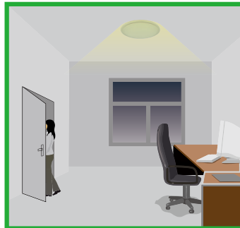
People left, light still dims to 0/10%/30%/50%(options) standby level after the hold time
