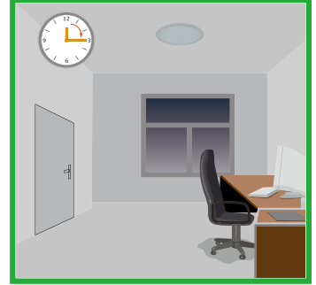
Light switches off automatically after the stand-by period elapses. (The light will keep stand-by level if preset the stand-by period is ∞)
