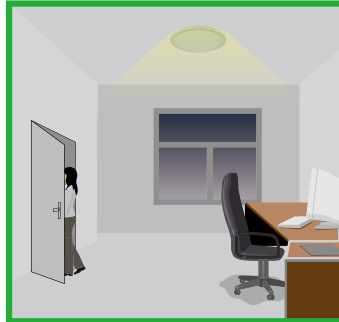
After hold-time, the light dims to stand-by level as preset dimming level.
