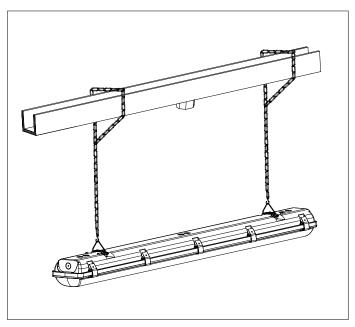
2.Secure mounting clips to housing recesses by firmly pressing them into place until both sides of the clip are secured.
