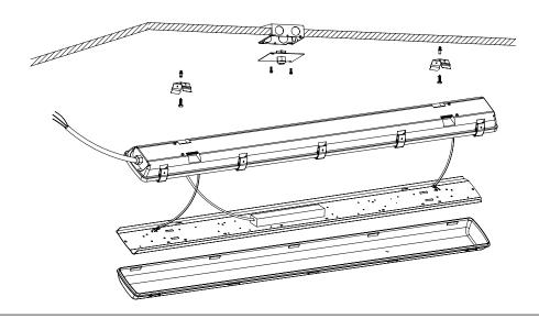
1. Screw two pieces metal bracket (packed in the accessory bag) to ceiling; install the housing to the metal bracket.
