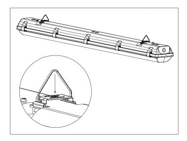
4. Release latches by pulling top of latch away from housing.
