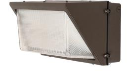
Luminaire utilizes long life, high efficacy LEDs and reliable LED driver. 120V-277V input voltage for increased versatility. Comes equipped with quick disconnect for compliance with US code. 0-10V dimming available.
