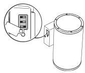
2. Replace the rubber cover securely to avoid water penetration into the fixture.
