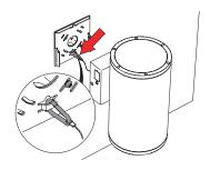
4. Secure the fixture mount to the quick mount plate using the screws removed in Step 1. Do not pinch any wires.
