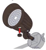
2. Replace the conduit plug securely to avoid water penetration into the fixture.
