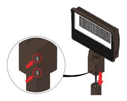
3. To aim the fixture, use a hex key to loosen the screw on the slipfitter. Rotate the fixture to the appropriate position and re-tighten the screw to secure it in position.
