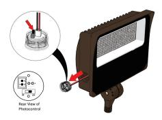
2. Replace the conduit plug securely to avoid water penetration into the fixture.
