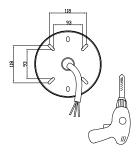
5. Remove the screws from the fixture base, twist the guick mount plate clockwise and separate it from the fixture base.
