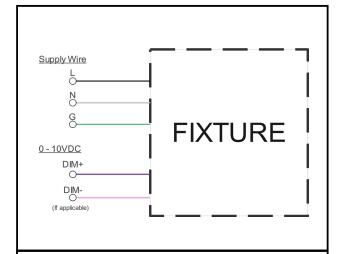
**Step 3:** Make the wiring connections according to the wiring diagrams on Page 4. Push excess wire into the junction box.
