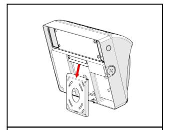
Step 4: Lift the fixture and tilt slightly toward the quick mount bracket. Hook the fixture housing onto the quick mount bracket as shown. Take care not to pinch any wires.
