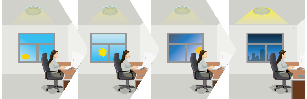
The light turns on at full or dims to maintain the lux level. The light output regulates according to the level of natural light available.
